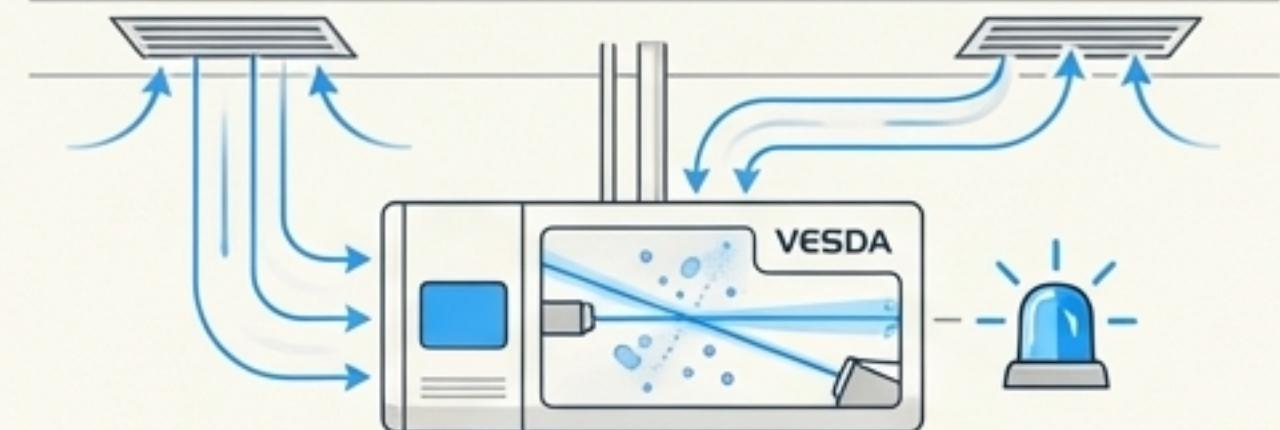
**Fire Detection:** VESDA (Very Early Smoke Detection Apparatus) continuously samples air for microscopic smoke particles, triggering alarms at the incipient stage of a fire, long before it is visible.
