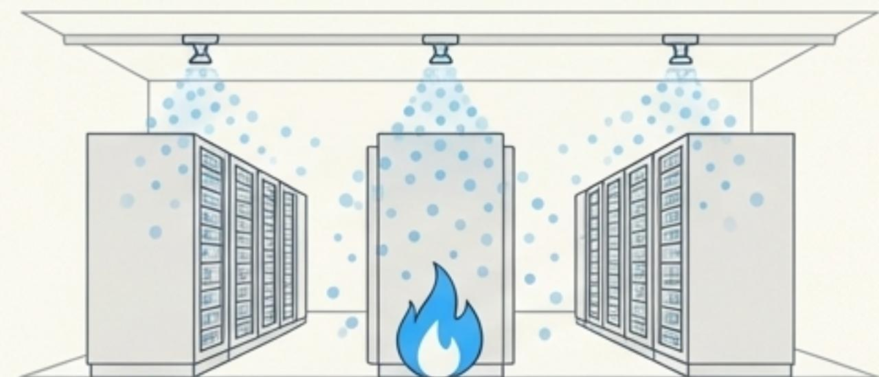
**Fire Suppression:** Clean-agent systems (e.g., FM-200, NOVEC 1230) extinguish fires with gas, causing no water damage to sensitive electronics. This preserves equipment and minimizes downtime.
